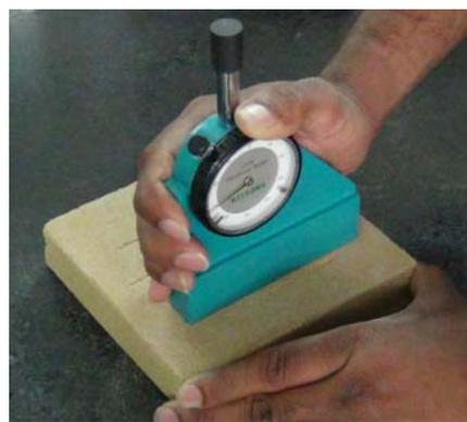
**Fig. 2: Mold hardness measurement**
