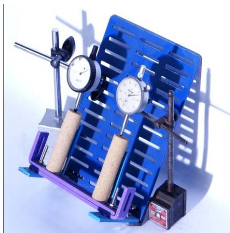
**Fig. 1: Core shrinkage measurement fixture**
